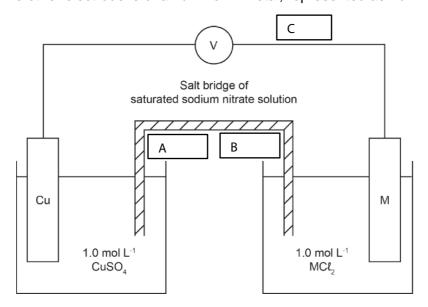
It was observed, that over time, the unknown metal electrode reduced in size and the solution containing MCl<sub>2</sub> remained colourless.
